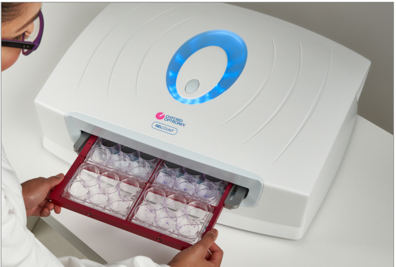
The GelCount: intended for processing adherent or 3D mammosphere colony formation assays
